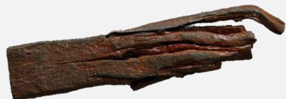
Wrought iron bar that was heated and the iron silicate hammered out.
